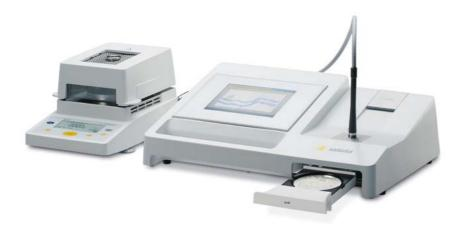
**Illustration:** The new LMA500 moisture analyzer from Sartorius, shown here with the MA35.
