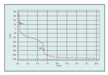
Titration curve for the determination of ephedrine hydrochloride according to method 6 (titration in ethanol with hydrochloride acid addition).
