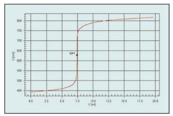
Titration curve for the determination of acesulfame potassium according to method 13 (titration in glacial acetic acid)
